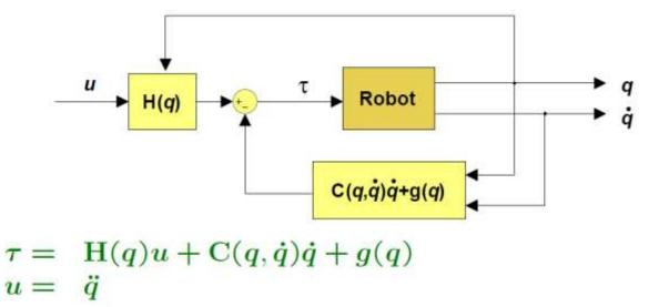
Due to compensation of nonlinearities and interactions in the close-loop the robot system is decomposed into independent subsystems and the control problem is reduced to a simpler problem of controlling independent linear systems.
