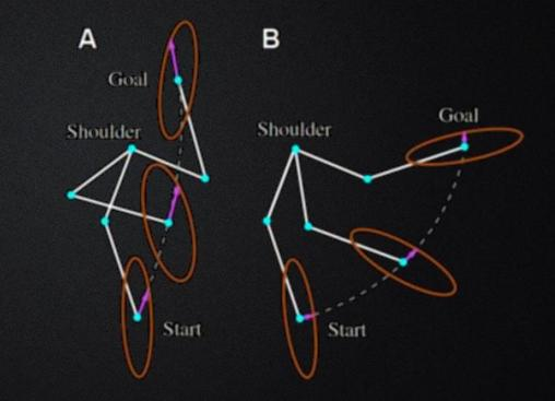
• The arrows represent manipulabilities in the given direction of motion.
