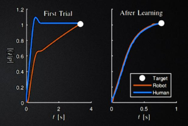
Adaptation of DMP weights for one subject during one session. The initial weights are in orange and the final weights are in blue. The intermediate steps are indicated with shades of gray. Comparison of human and robot trajectories for the initial trial (left plot) and trial after the finished adaptation of the movement profiles and Fitts' law parameters (right plot).
