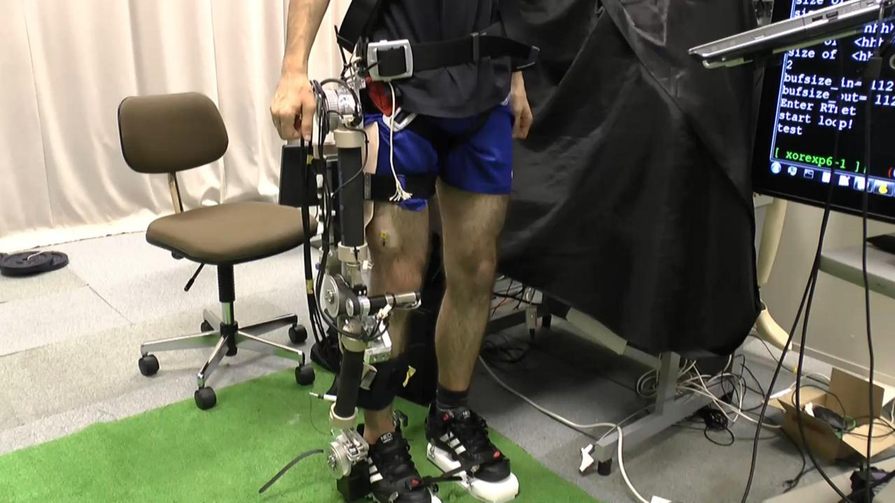
Neuromechanical modeling is a powerful tool that can be successfully used as the underlying basis for controlling exoskeletons.
